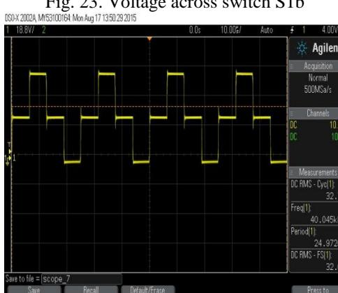
Fig. 24. Voltage across switch S2a
