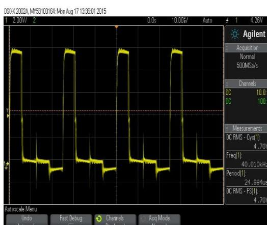
Fig. 20. Pulses for switches S1a and S1b
