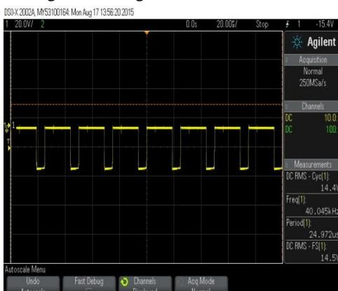
Fig. 26. Voltage across diode 1
