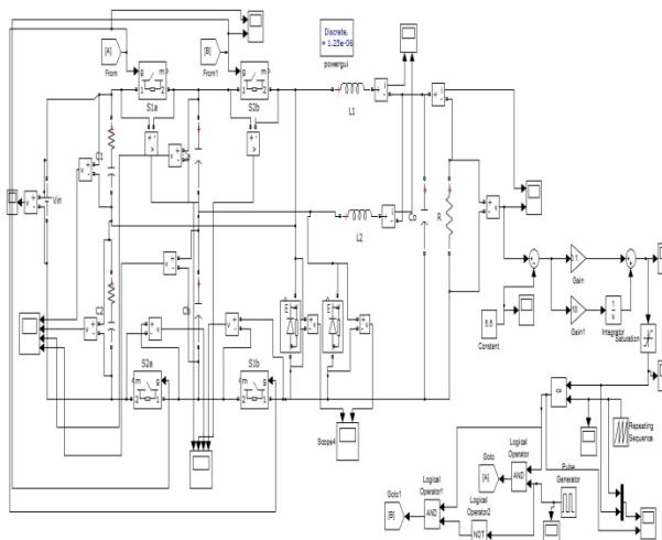
Fig. 8. Simulink model of the closed loop operation
