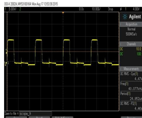
Fig. 21. Pulses for switches S2a and S2b
