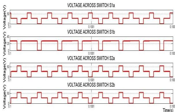
Fig. 13. Voltage across the switches
