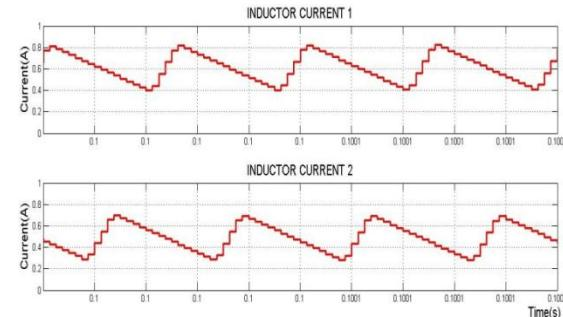
Fig. 14. Current through the inductors
