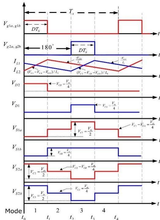
Fig. 4. Key operating waveforms of the new IBC
