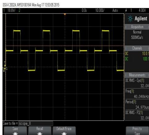
Fig. 25. Voltage across switch S2b
