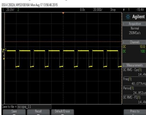
Fig. 27. Voltage across diode 2
