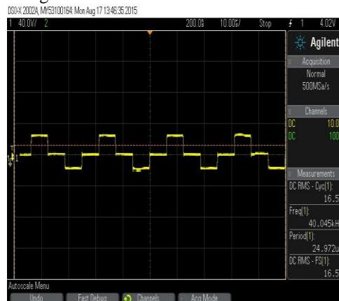
Fig. 22. Voltage across switch S1a
